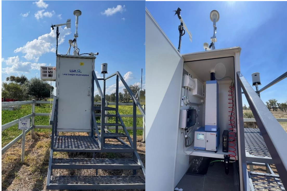
Figure 1: TEOM installed at Lanreef
